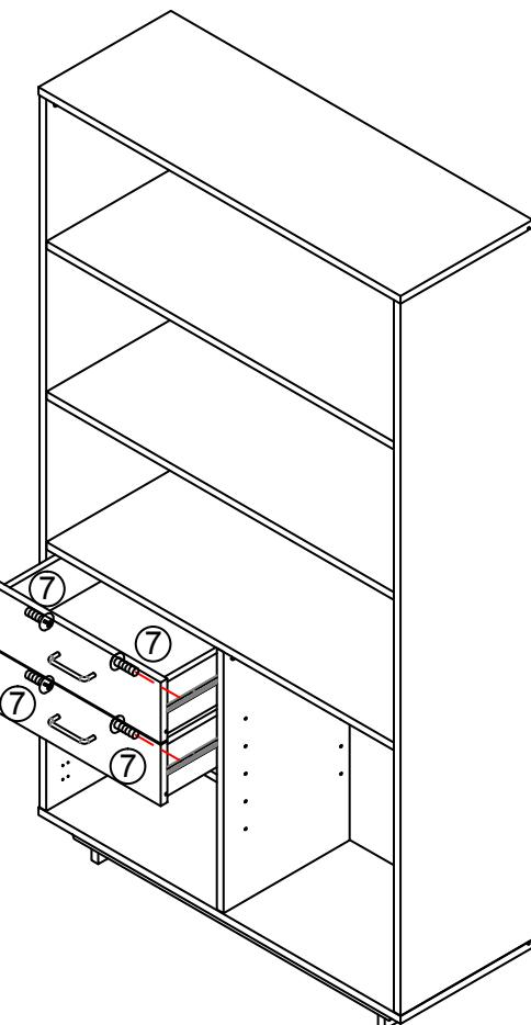
Align side drawer rails to the hole of the drawer sides. Secure by using bolts (#7).
