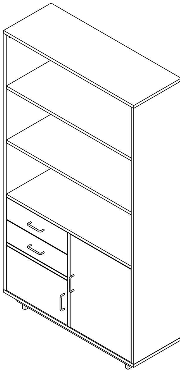
Make sure the unit is rested on a flat surface and does not feel loose or wobbly. If it does, double check all bolts/screws are secured and properly tightened.
