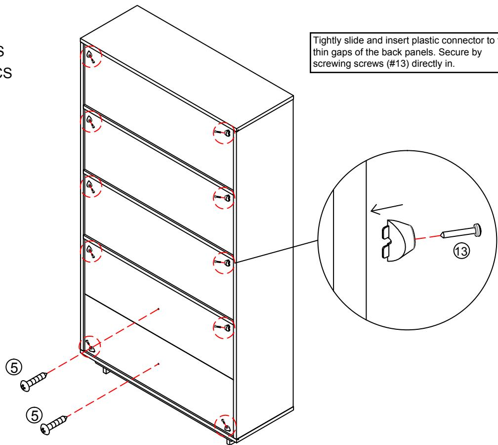
Tightly slide and insert plastic connector to the thin gaps of the back panels. Secure by screwing screws (#13) directly in.
