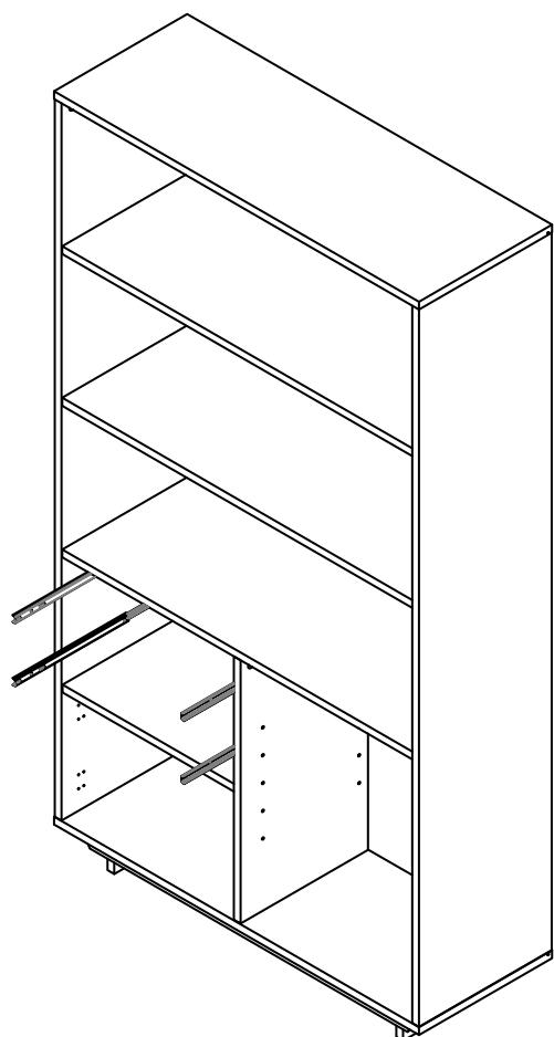
Please press the slide firmly while fixing the screw on the side panel of drawer.
